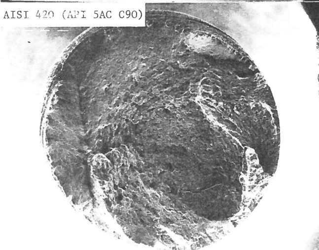
Fig. 7 - Macro and micro fractographies of smooth specimens.
