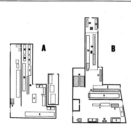
Fig. 1. Plating room layout before (A) and after (B) the reorganizing operation. Plant identification is given in Table III. In part A also shown are the plant and equipment not related to the plating room and subsequently moved, while in part B the plants and equipment which have been added and the areas (I, II, III) which have been isolated are stressed.
