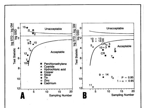
Fig. 2. Contaminant sampling results before (A) and after (B) the plating room reorganization: application of the OTL (one-sided tolerance limits) decision criteria. For plant identification and symbol key see Fig. 1 and Table IV.
